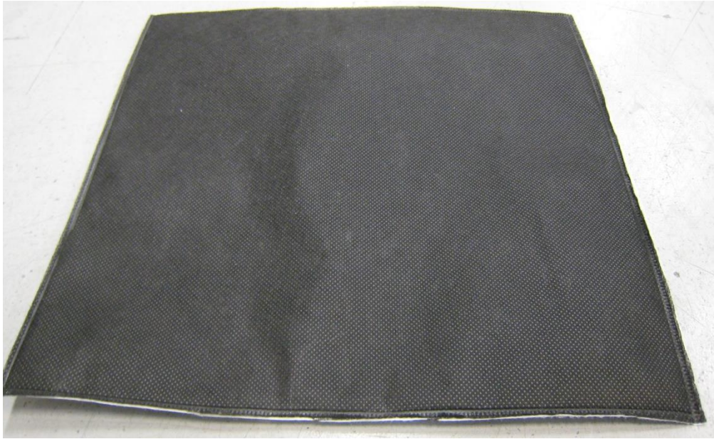
Fig 1. Overview of the filter material (upstream).
